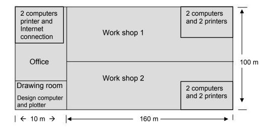
The four computers and their respective printers used for computer-aided manufacturing (CAM) are located in the workshops. These computers and printers need to be mobile, as they are moved to where other, larger equipment is located. The computers are shielded against electro-magnetic interference produced by nearby welding equipment.
